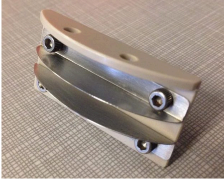
Figure 5.11: (Left) A capacitive level meter to hang alongside the TPC. (Right) A test of the capacitance rise with the insertion of a PTFE card.
