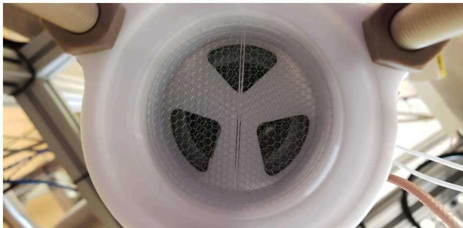
Figure 7.3: A view of the TPC active region from below, with the source rod installed.
