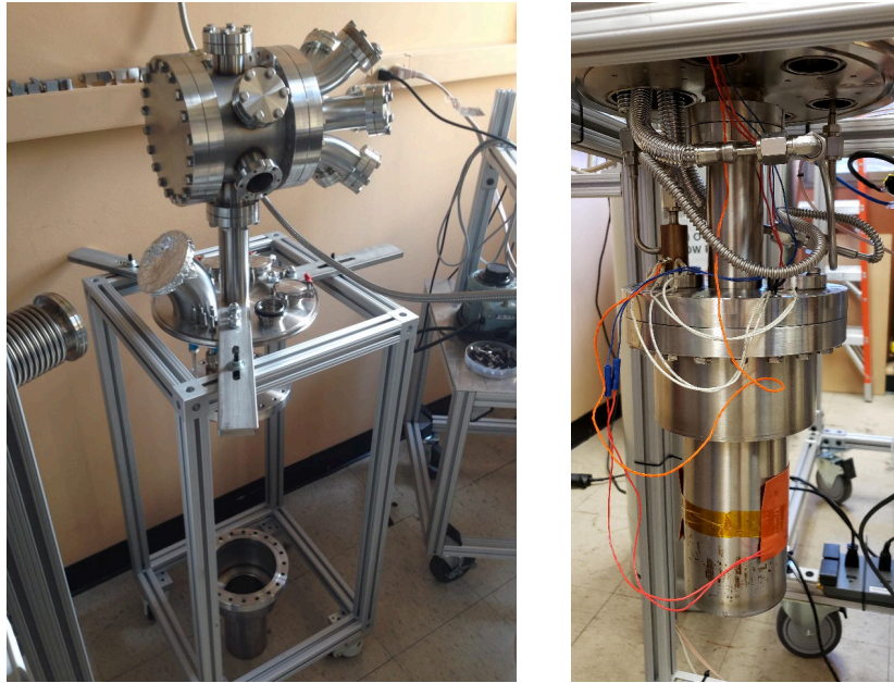
Figure 5.18: (Left) The Medusa head mounted on a T-slot frame, with cabling pipe extending down into the cold space. (Right) Inner vessel can sealed up, enclosing the Xe space.
