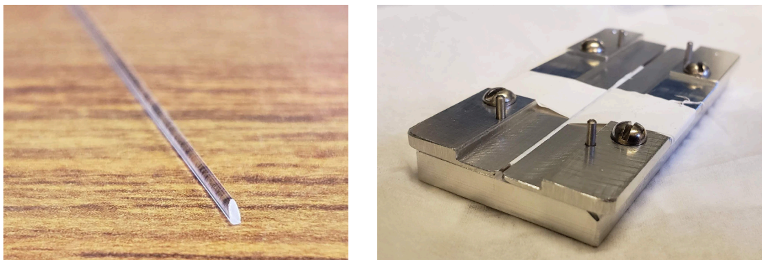
Figure 7.2: (Left) An example fused silica rod with a beveled end. (Right) The metal jig clamping down on a masked fused silica rod before source deposition.
